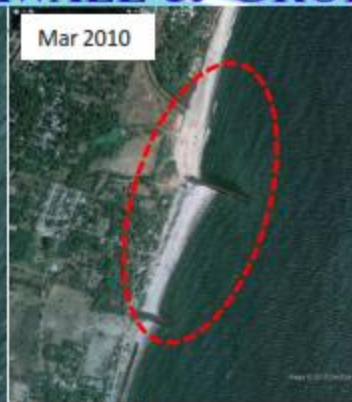
2 km length of coast line protected by both seawall and groins by Tamil Nadu
