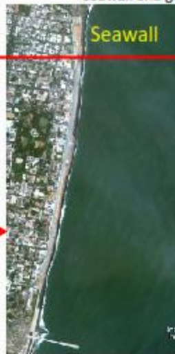
2 km length of coast line protected by both seawall and groins by Tamil Nadu
