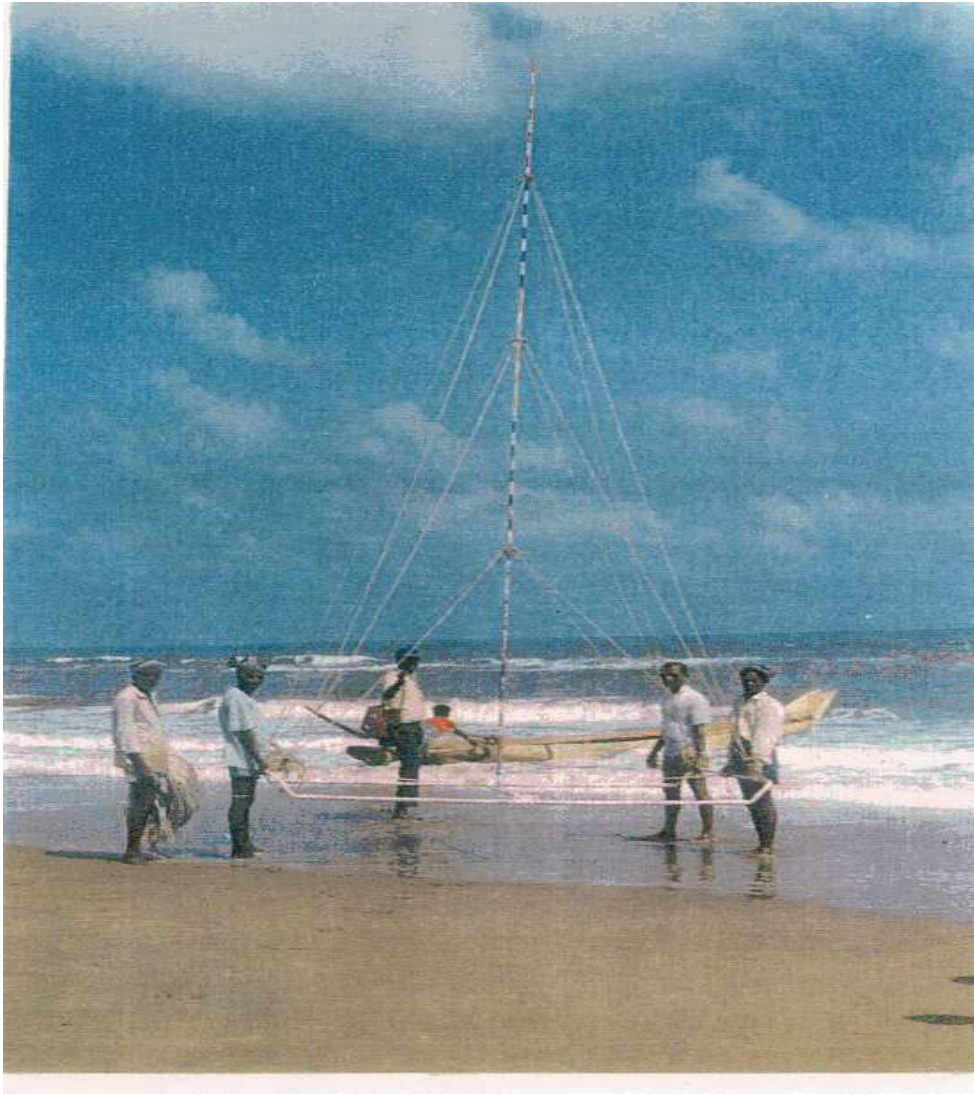
Figure 3.1.1 Near-shore profiling using wave sled
